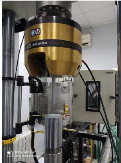
Fig. 1. General view of the fixing device installed on the Instron 8802 testing machine.
