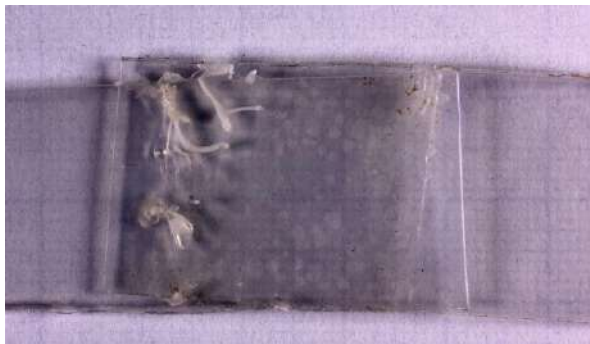
Fig. 2. Ultrasonic overburden weld of biodegradable film made of sonotorod with a flat surface.
